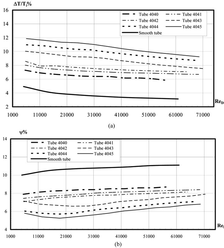
**Figure 8** Percentage of feed water temperature raise ratio and exergy destruction rate for a three-start spirally corrugated tubes (ridge height = 0.781 mm) with twisted tape presented by Zimparov (2001) at  $T_s = 328.8$  K,  $T_o = 298$  K and  $T_i = 2901$  K. (a) Percentage of feed water temperature raise ratio and (b) Percentage of exergy destruction ratio
