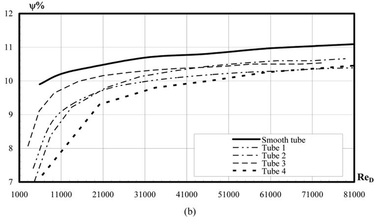
**Table 5** Percentage of feed water temperature raise ratio and exergy destruction rate for spirally corrugated tubes studied by Zimparov et al. (1991) at  $T_s = 328.8$  K,  $T_o = 298$  K and  $T_i = 290.1$  K
