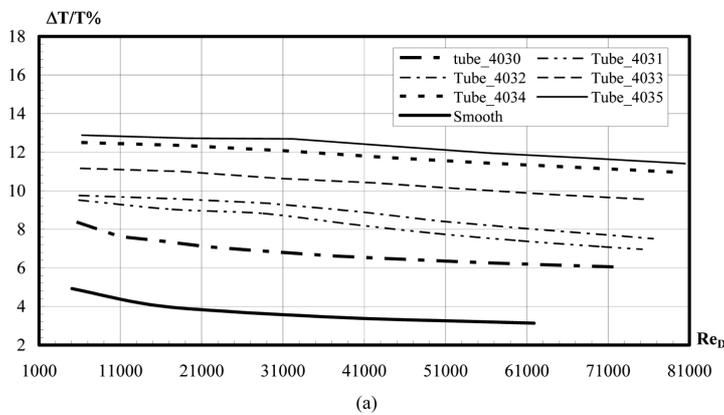
**Figure 8** Percentage of feed water temperature raise ratio and exergy destruction rate for a three-start spirally corrugated tubes (ridge height = 0.781 mm) with twisted tape presented by Zimparov (2001) at  $T_s = 328.8$  K,  $T_o = 298$  K and  $T_i = 290.1$  K. (a) Percentage of feed water temperature raise ratio and (b) Percentage of exergy destruction ratio (continued)
