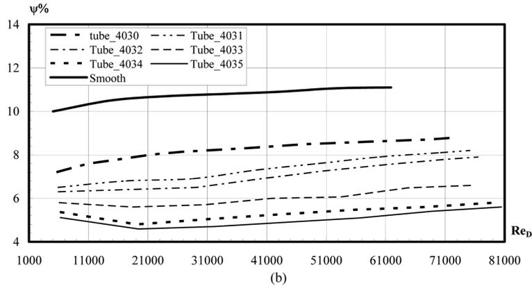
**Table 6** Percentage of feed water temperature raise ratio and exergy destruction rate for different discussed tubes at  $T_s = 328.8$  K,  $T_o = 298$  K and  $T_i = 290.1$  K
