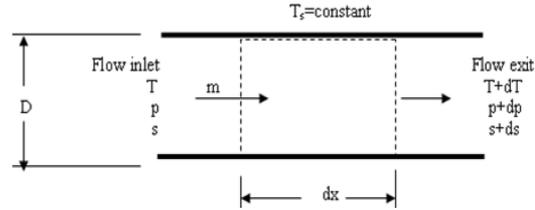
Also, the percentage exergy destruction rate associated with the heat transfer process along the duct can be calculated by,
